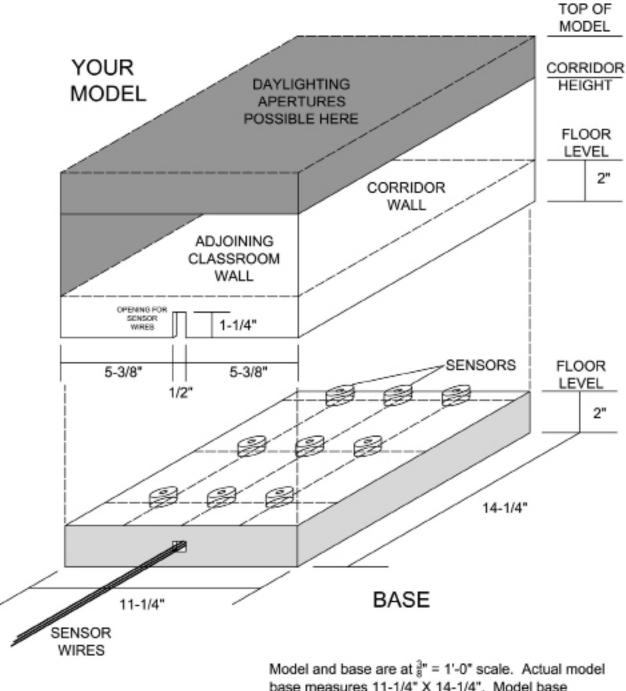
Model and base are at  $\frac{3}{8}$ " = 1'-0" scale. Actual model base measures 11-1/4" X 14-1/4". Model base thickness is 2" high. Remember to ADD this height to model walls.
